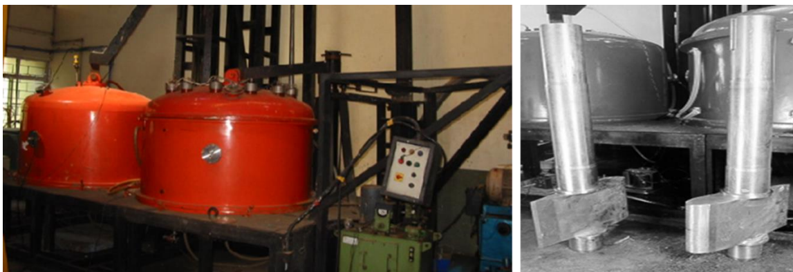
Figure 1: Plasma nitriding system to treat large components such as Guide Vanes
