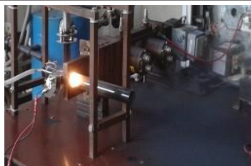
Vishal's Torch : Microwave plasmas are warm plasmas. They have much higher electron temperature compared to DC or RF plasmas
