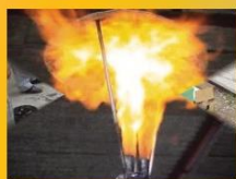
Quality of pyrolysis gas is checked by intensity of flame
